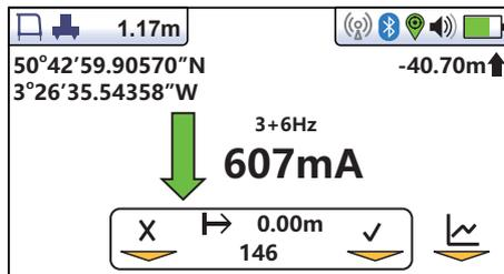
Pressing the "Enter" key will save the DM current shown with the saved A-Frame results.
