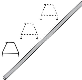
Note the depth of the pipeline. Move approximately this distance to one side. Keep the orientation as the above walk along the section of the pipeline taking readings at regular intervals. A typical result is shown below with the main defect being the largest reading. Note that the arrow will always point to the pipe, i.e., will not reverse unless the signal reduces to a level that cannot be processed correctly.
