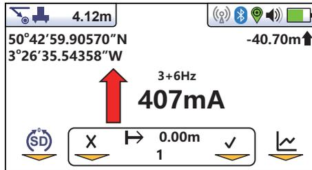
A short press of the On/Off pushbutton will synchronize the system and return the unit to the locate screen. The green forward arrow will light and not be flashing indicating the receiver is locked onto the signal. The system is now synchronized.
