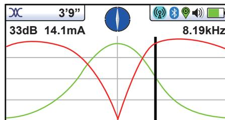
To take a plot, first locate the target using one of the other locate screens. Now select the Transverse screen by a prolonged press of the return button. Repeat this until the Transverse screen appears.
