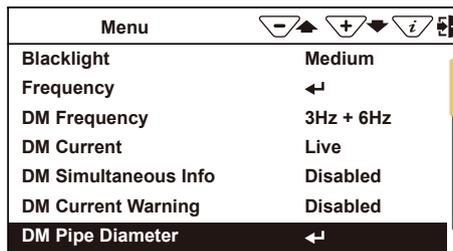
Use the “Enter” key to enable the diameter of the pipe to be entered.
