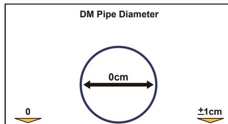
A short press of the On/Off key sets the diameter to zero, which effectively switches off the depth of cover feature and measurements are then to the center of the pipe.
