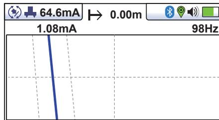
“Tram” lines either side of the line indicate an area of confidence. The closer the tram lines are together, the greater the confidence.
