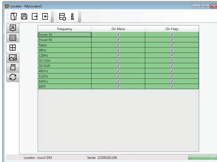
The “Frequencies” page will allow the user to refine which frequency modes are available when the locator F-key is pressed and which frequencies appear on the locator menu.
