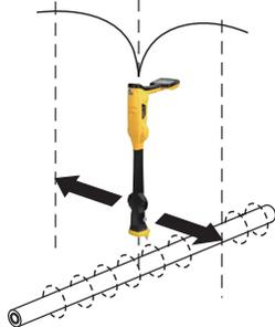
This uses dual vertical antennas. This has the advantage that it provides a sharper response than the “null” mode and is less affected by distorted fields. All other functions are the same as the “Null” mode.
