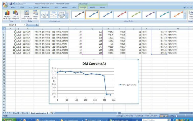
The graph is drawn with a linear current x-axis. If a logarithmic scale is required, right-click on the x-axis and select logarithmic from the options as below.
