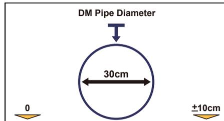
Use the “+” and “-” keys to enter the desired value. Note that entering the incorrect value will result in a depth of cover indication error.
