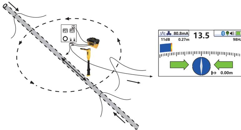
Keeping the receiver pointing at the connection point, walk around the connection point for a full 360 degrees. The reading on the receiver signal strength meter will rise and fall as it passes over:
