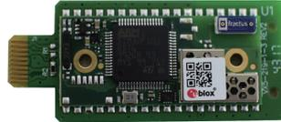
The vLoc3-DM receiver can be fitted with an optional Bluetooth communications accessory. This allows communication with external GPS and or Dataloggers. The Bluetooth option can be retrofitted and can be ordered at a later date if preferred.
