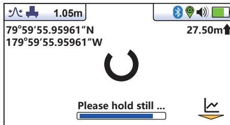
After approximately 2 seconds, the rotating circle and progress bar will be replaced with the result display as below.
