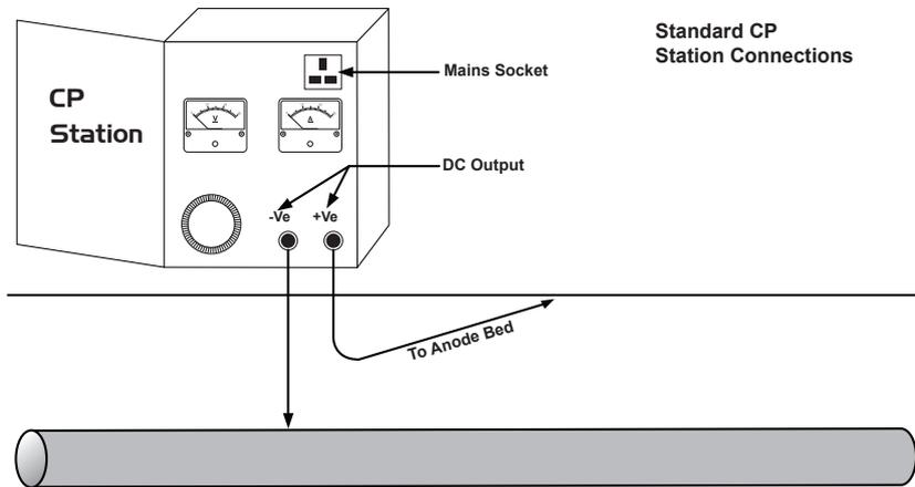
3. Disconnect the output wires connecting the CP station to the pipeline and anode bed. If there is an earthed mains socket at the station, connect the transmitter mains power lead to the socket.
