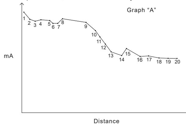
Also, note the step response at points 1 to 2. This is typical of readings near the application point and may not represent a fault. The step is very often caused by the concentration of ground currents at the application point or the cable leading to the ground bed. If in doubt, check the section using the A-frame.
