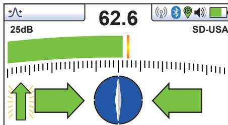
Re-trace your line back to a point where a solid signal direction is obtained. Precisely pinpoint the line and stand with your back to the direction of the transmitter as you did when you initiated the original sync and press the "i" pushbutton, then a short press of the pushbutton to re-sync with the transmitter signal.
