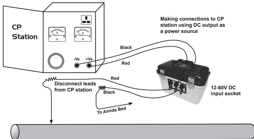
5. Adjust the transformer output to approximately 40V DC (although the unit will function from 12V DC to 60V DC) and use the DC input lead to connect the transmitter to the transformer terminals.
