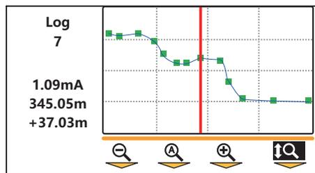
If the operator walks back along the pipeline, the cursor will alter, indicating the position of the operator. This allows the operator to return to the point of interest without having to repeat the survey.
