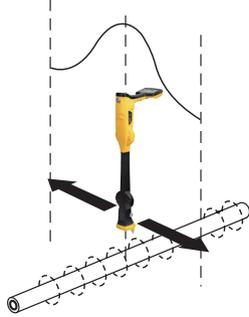
The peak with arrows mode operates in the same way as the peak mode. It gives the largest meter deflection when directly over the line. However, Left/Right indication arrows are also displayed. The arrows indicate the direction to move the receiver to locate the position of the buried line.
