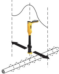
Two horizontal antennas provide a “Peak” or maximum signal response over the center of the buried line. The compass (line direction indicator) aligns itself parallel to the direction of the cable (available in Active modes).
