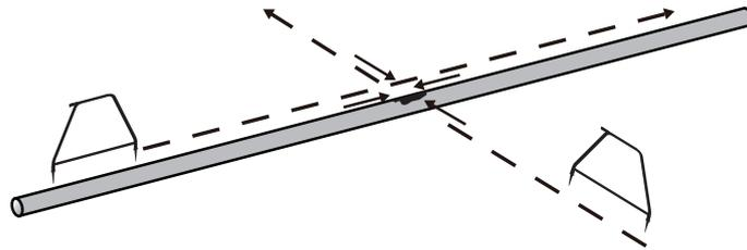
Sometimes it is not possible to gain access to the pipe position. If this is the case walking along the route of the pipe a few meters to one side can very often produce good results. This procedure is also useful where the pipe runs under “blacktop,” which acts as an insulator preventing the A-frame from making a good connection to ground.
