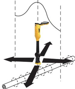
When you see the two double-ended arrows around an icon, this means that the line is detectable regardless of locator blade orientation. It is very useful for quickly checking an area for buried lines using a grid search as one sweep will catch all locatable lines. In the classic screen, the Omni feature is available in the “Peak” and “Broad peak” modes.
