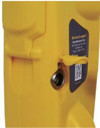
Connect the charger to the charging/accessory socket of the receiver. Connect the charger to the mains and switch on. The LED indicator on the charger will illuminate red until the batteries are fully charged, at which time the LED will change to green.
