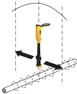
This uses a single horizontal antenna and provides a “Peak” or maximum signal response over the center of the buried line. The compass (line direction indicator) aligns itself parallel to the direction of the cable (available in Active modes).
