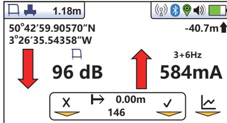
Pressing the "Enter" key will save both A-frame and DM current readings.
