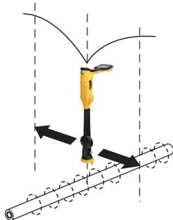
This uses vertical antennas, and provides a minimum or “Null” response over the center of the buried line.
