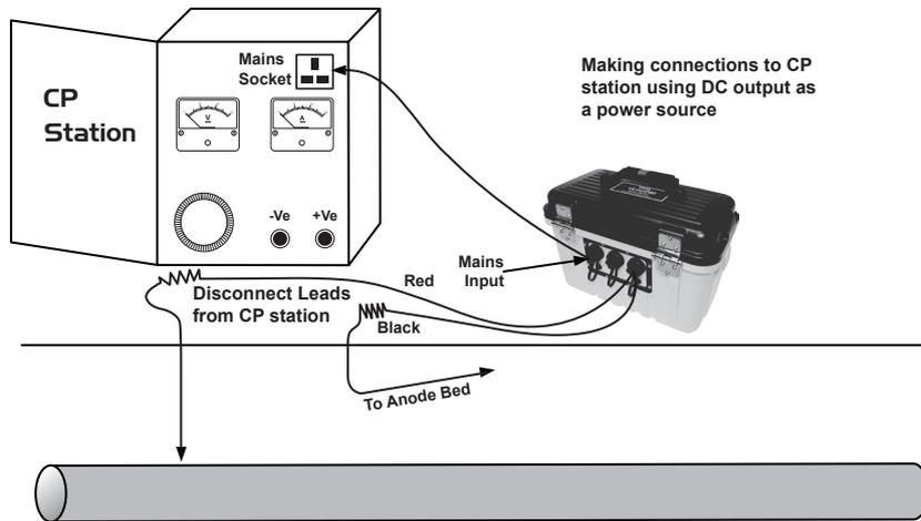
4. If there is no mains socket, it is possible to use the DC output of the transformer rectifier. See the diagram below.
