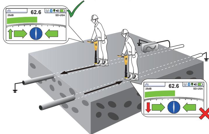
At some point you may find that the SD arrow starts to flash. This is indicating that synchronization with the transmitter has deteriorated and a reset is required.
